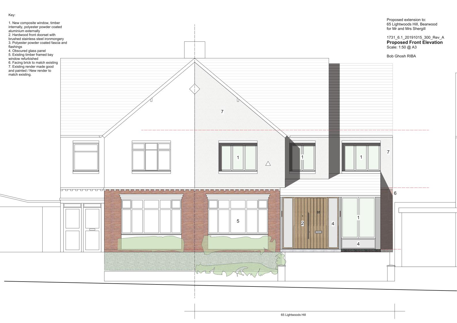
1. New composite window / French window, timber internally, polyester powder coated aluminium externally
